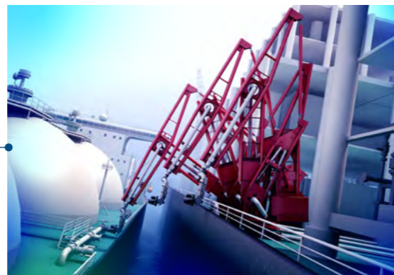
OLAF Offshore Loading Arm Footless
