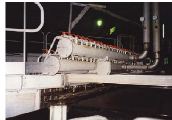
CLOTH AND TABLE WASHING The cloths are cleaned under pressure by two spray banks fed by one or two central manifolds. Residual gypsum is removed and cloths and table are washed to prevent scaling.
