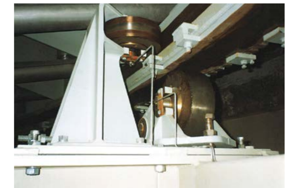
SUPPORT AND CENTERING ROLLERS Filter frame is supported and centered by sets of rollers mounted on nodular cast iron supports
