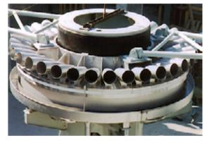
**FILTER VALVE**The upper part of the filter valve is easily raised for fast inspection or adjustment
