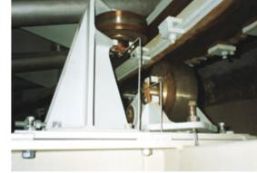
**SUPPORT AND CENTERING ROLLERS**Filter frame is supported and centered by sets of rollers mounted on nodular cast iron supports
