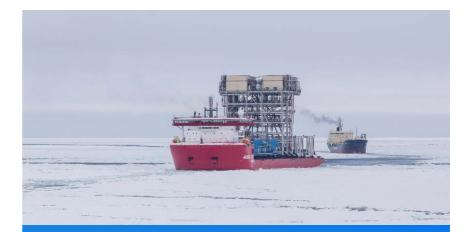
Technip Energies and its partners confronted the site's freezing and isolated conditions by choosing a modular construction approach, contracting with 10 Asian fabrication yards to build 142 modules and 365 pre-assembled pipe racks weighing more than 480,000 tonnes. Yamal LNG became one of the largest modular construction projects in the world.
