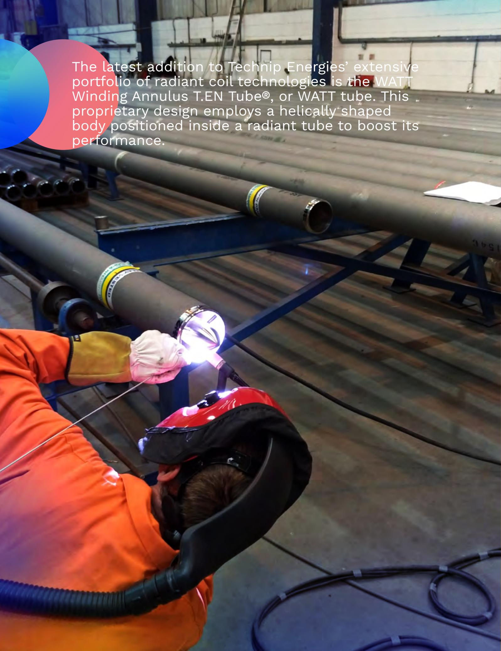
The latest addition to Technip Energies' extensive portfolio of radiant coil technologies is the WATT Winding Annulus T.EN Tube®, or WATT tube. This proprietary design employs a helically shaped body positioned inside a radiant tube to boost its performance.
