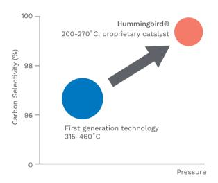
Hummingbird is a second generation, low-cost process for dehydrating ethanol to ethylene. The technology uses a proprietary heteropolyacid (HPA) supported catalyst, operating at a lower temperature, higher pressure, and higher selectivity than first generation processes.
