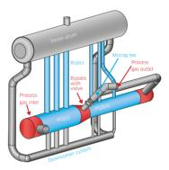
Our company developed process gas boiler includes a two chamber design for enhanced overall heat transfer, and an external bypass assembly to ease both operational and maintenance requirements.
