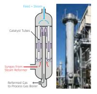
The Technip Energies' Parallel Reformer TPR® is our proven convective recuperative reformer, also suitable for retrofits. It is designed to optimize the high-grade heat utilization and increase reforming capacity without additional firing, thus resulting in lower CO<sub>2</sub> emissions by up to 20%.
