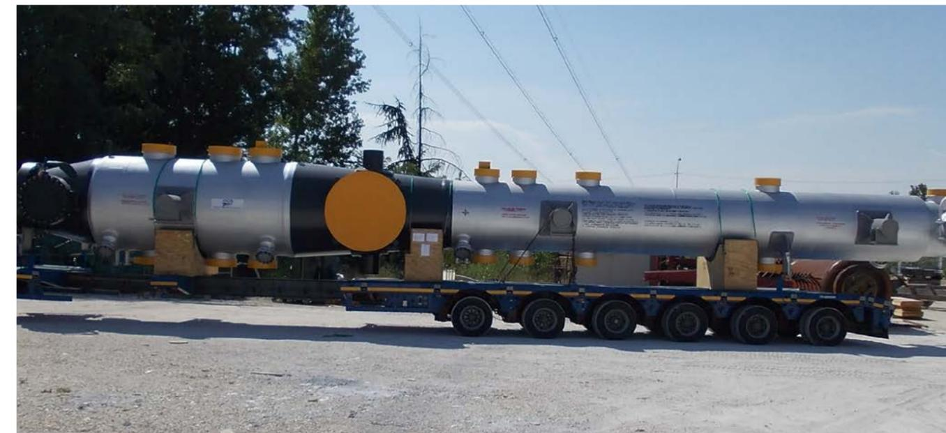
Transportation of a process gas boiler to the plant site
