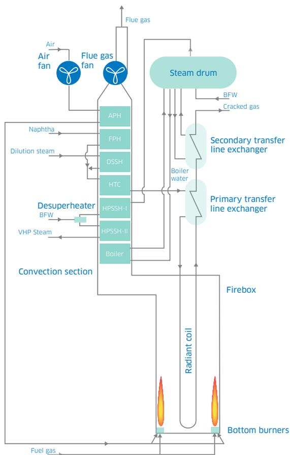
Fig. 1. Low-emission cracking furnace with air preheat.
