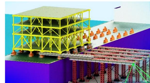
After completion of skidding and jacking down operations, the skid deck elements are retrieved onshore
