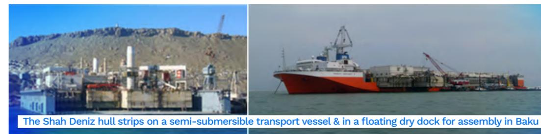
The Shah Deniz hull strips on a semi-submersible transport vessel & in a floating dry dock for assembly in Baku
