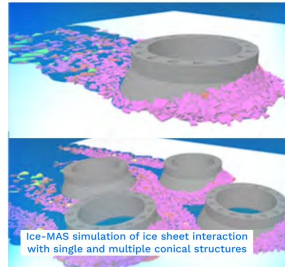
Ice-MAS simulation of ice sheet interaction with single and multiple conical structures
