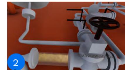
2: The fluid nature and velocity in the transparent pipeline is computed in real time by the dynamic process model and animated in the physical simulation.
