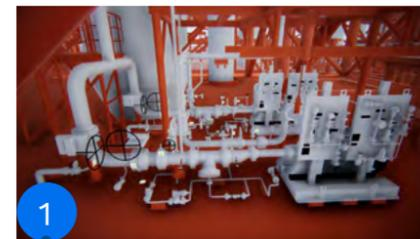
1: Field equipment such as manual valves actuated in the physical world simulation by the operator in VR are transferred and taken into account in the dynamic process model.
