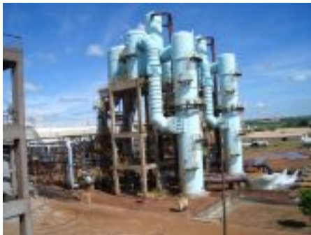
Large capacity concentration units (1,100 tpd evaporated), MOSAIC Brazil, Uberaba, Minas Gerais, Brazil
