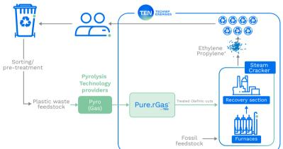
Pure.rGas purification and upgrading train ensures adequate feed preparation that enables a safe cracker integration. The design is flexible to different pyrolysis technologies and to any kind of crackers (gas or liquid cracker / front-end or back-end hydrogenation scheme). The selected process scheme benefits from:
