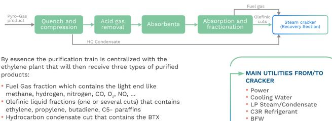
Hydrocarbon condensate cut that contains the fraction
