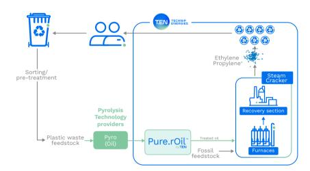
Our proprietary Pure.rOil purification and upgrading train ensures safe and flexible feed preparation for any liquid cracker. This technology benefits from:
