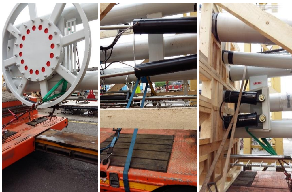
Figure 6: Example of lashing for a Loading Arm
