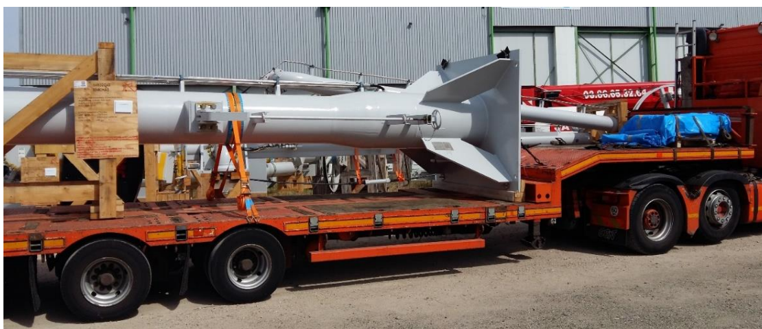
Figure 7: Examples of lashing for a Base Riser
