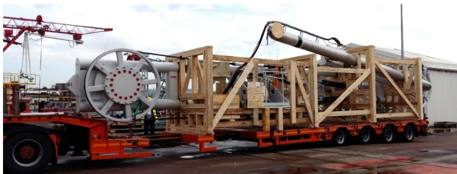
Figure 5: Example of extendable truck with perpendicular bar
