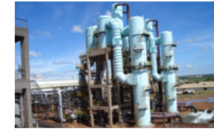
Large capacity concentration units (1,100 tpd evaporated), MOSAIC Brazil, Uberaba, Minas Gerais, Brazil
